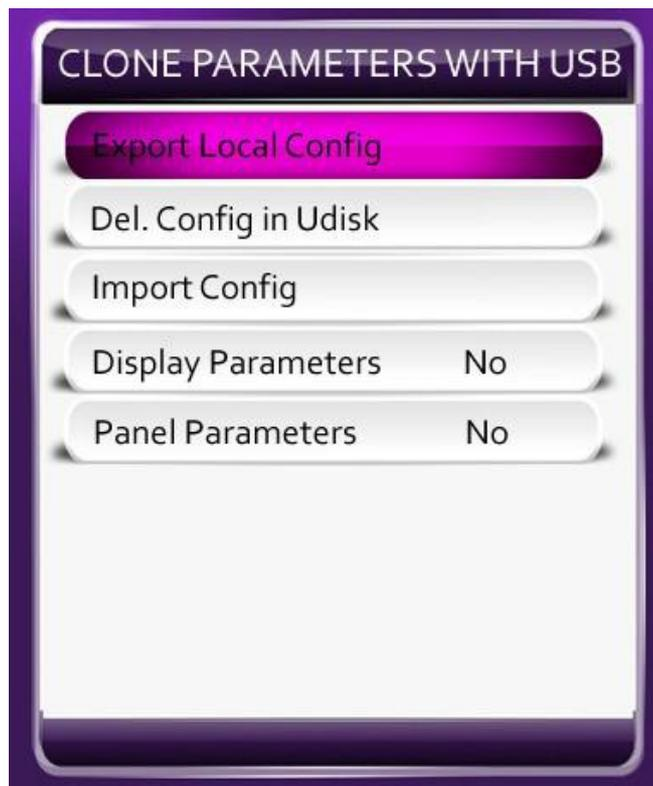
1. Export Local Config: Set local system configuration to the file named “T10\_usb\_setting.txt”, and copy it to the USB.
