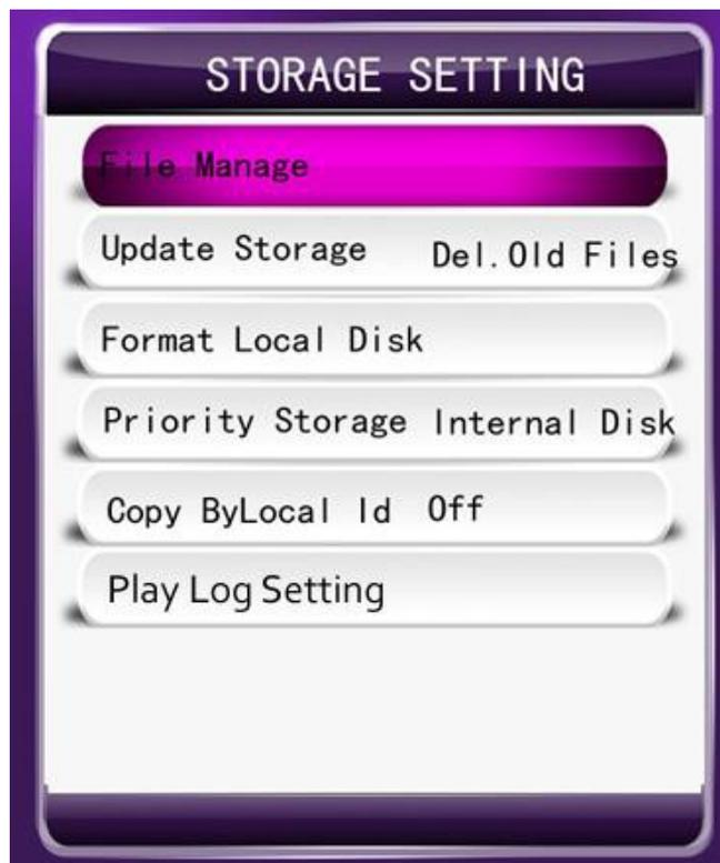
1. File Manage: This allows you to view the files in storage. Use the remote to navigate and select a file. Press the play button to play the file or DEL to delete the file.
