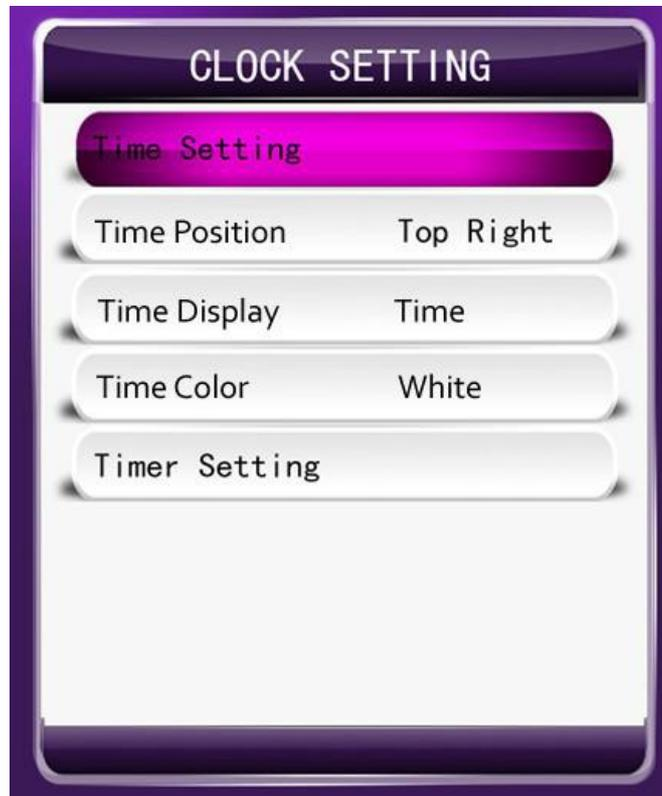
1. Time Setting: Set the time of the machine and press “Save The Time” to update.
