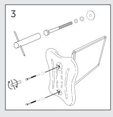
Use the fixings shown to attach the water-fillable base to the frame.
