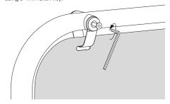
B Locate panel onto the panel hanging clips. Reassemble the panel hanging clips using the screws and fixings.
