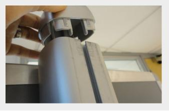
2. Use Allen key to loosen the widget to fit into the channel
