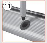
Close the main body cover. Open the telescopic pipe and embed it to the hole on the body.
