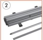
Turn the feet 90 degrees as in photo, then open the cover profiles of the base and take out clips profile  $\delta$  telescopic pipe.
