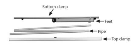
Form the base into a "T" shape and fix in position by turning the plastic connector.
