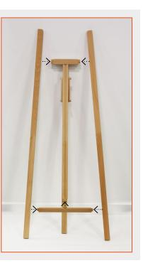
2. Place on a flat surface, ensuring the holes on the back of the T section and cross member are facing upwards. Insert a brass locator into one of the T section holes and position using a slotted screwdriver. Screw 1 medium brass bolt through the side of the leg into the T bar using a Phillips head screwdriver, ensuring it threads through to the locator insert. Repeat to secure the legs to the other side of the T section and the crossmember.
