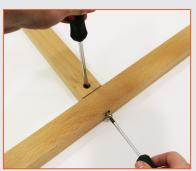
**5.** Take the T section and ensure that the metal ratchet is facing downwards. Align the holes at the top of the T section with the holes at the top of each of the legs and secure them using 2 brass screws and a Phillips head screwdriver.
