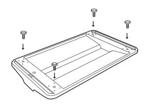
Screw in the eight Allen screws to securely fix the screen and the base together
