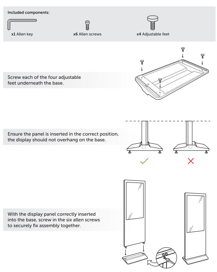
**Underneath base:** x3 screws per side (x6 screws in total)
