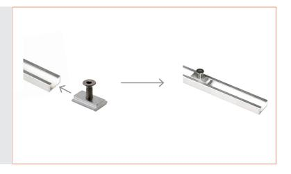
2. Fit your cable and fixings (e.g. AA4) or rod and fixings (e.g. ARG05 and ARG06) onto the top of the screw supplied with the toggle (AH03).
